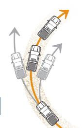
**StabiliTrak.** The StabiliTrak Electronic Stability Control System with Traction Control helps you avoid what the road might throw at you by improving vehicle stability, particularly during emergency maneuvers.
