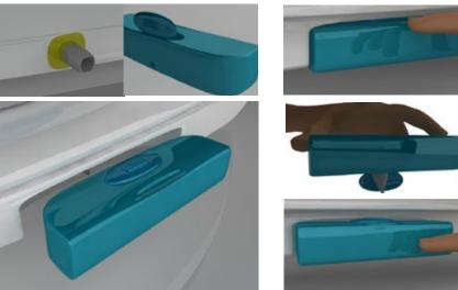
Calc - Clean System Integration: (Based on utilizing Phillips Calc Cleaning System) Once the calc clean process is completed inside the heating compartment, the Calc is collected through a metal connector to a detachable plastic container located on the lower right hand side of the base unit. The user can then remove the Calc container and open it for easy disposal.
