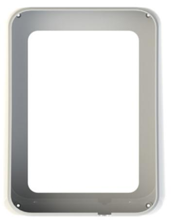
The mid piece of the casing is white, Injection Moulded, recyclable ABS and attaches to the back piece. The monitor rests on it to allow it to be attached to the front piece. The mid piece first screws into the front piece to secure the monitor into position and is then screwed to the back piece.
