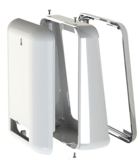
The Casing of the Shower touch would be manufactured with three separate pieces and incorporate two splitlines. When packaged the middle section and front section would already be assembled but they would not be fixed to the back section allowing the user/ plumber to construct any additional piping to the mains required. This also allows the back of the shower Touch to be screwed to the wall.
