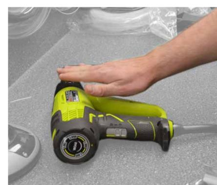
Once the user is done using the heat gun, the metal tip will stay hot for a long time, preventing the user from storing it away.
