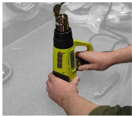
The Ryobi heat gun was not very stable when it was sitting on its end, this was extremely onconvenient for bending pipes.
