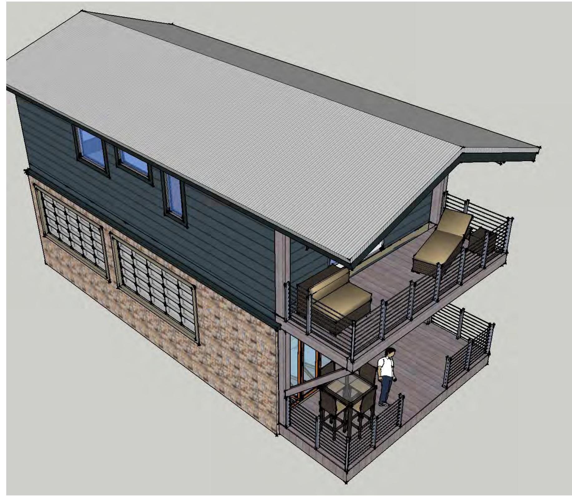
METAL ROOF NON PAINTED ACRYLYC COATED GALVALUME
