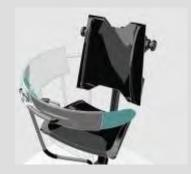
UNO has a wide vision spectrum in the front to help reducing the "blind spots" typically found in a regular vehicle. The windshield makes up 30% of the totalstructure and is the main access to the vehicle.
