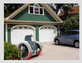
The vehicle has an exterior chassis that resembles the exoskeleton on the outside of the insect's body. In addition, the chassis is build of detachable panels made of recycled materials (PET).
