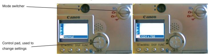
Verify that settings on individual AE cameras are correct by setting the mode to **Auto** or . Press FUNC. and check to see that the bottom of the display reads **Normal** (this is the compression). If not, scroll left/right with the control pad until it is set. Press down on the control pad to change the resolution, and set this to **1024 x 768** by moving left/right.
