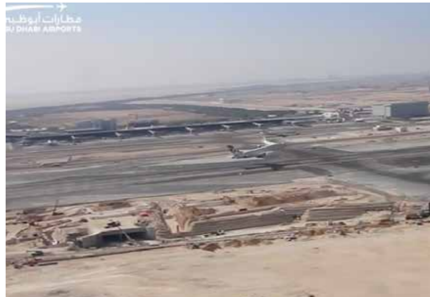
The location of the Terminal Building between the two main runways allows for more efficient ground operations and taxiing time, whichever runway is used.
