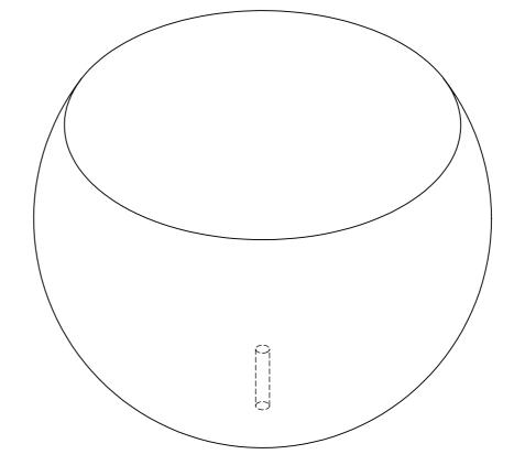
SPHERE SCREWS DOWN ONTO THREADED SUPPORT BAR
