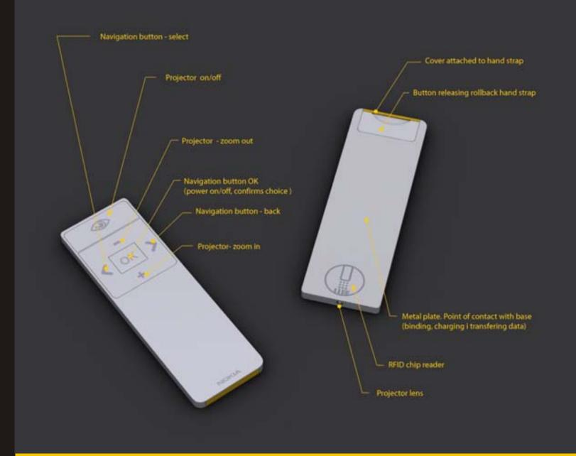
SCHEMATIC VIEW AND DESCRIPTION OF PORTABLE PART
