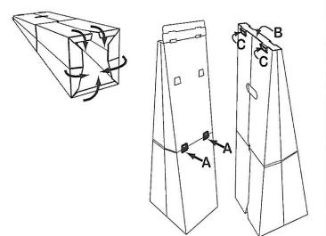
2 A) Insert two S CLIPS on MIDDLE set of slots on Tray without Riser.
