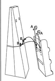
3 A) Insert two S CLIPS on MIDDLE set of slots on Tray with Riser.
