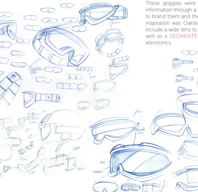
These goggles were designed to provide safety information through a HEADS UP DISPLAY. We had to brand them and the company I chose to use as inspiration was Oakley. The main design features include a wide lens to increase peripheral vision as well as a SEGMENTED band design to house the electronics.
