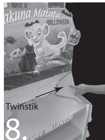
8. Remove covering from Twinstik on flanges where shown. Fold back and adhere to hutch.
