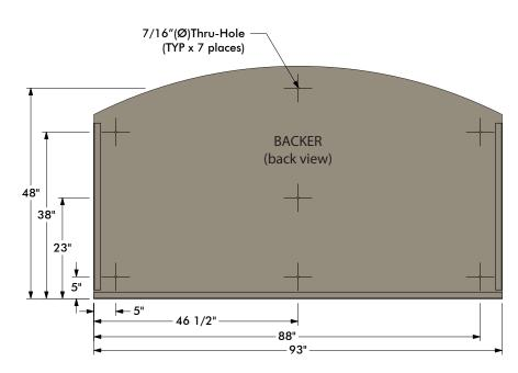
NOTE: Backer & support angles welded to back of backer
