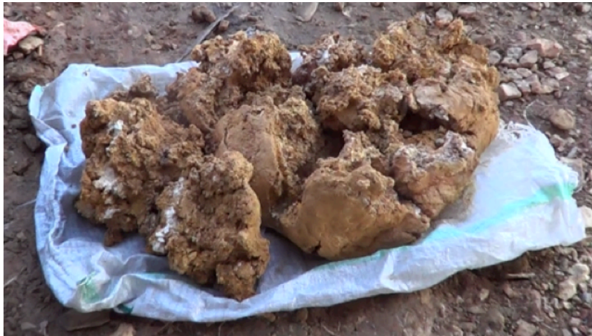
Figure 7. Ore material for documentation. Two sacks of gawds, a type of ore commonly found in Aroroy, Masbate) were used. This particular sample contains 1 gram of metal, based on the assay done prior to the documentation process.
