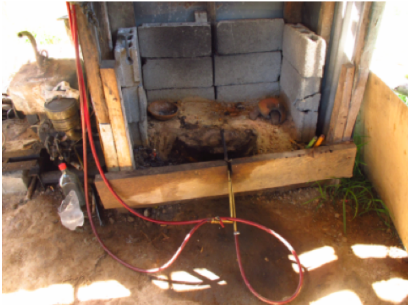
Figure 6. Furnace set-up. Acetylene blowtorch is used to smelt the metal concentrate with borax. Ceramic pots are used during smelting because of its capacity to tolerate high temperatures.
