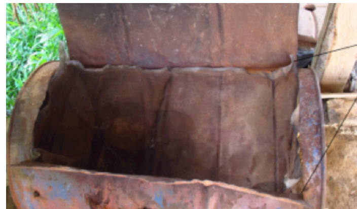
Figure 5. Improvised Grill. Old rodmills are recycled and used as grills for burning the activated carbon using coco shell charcoal
