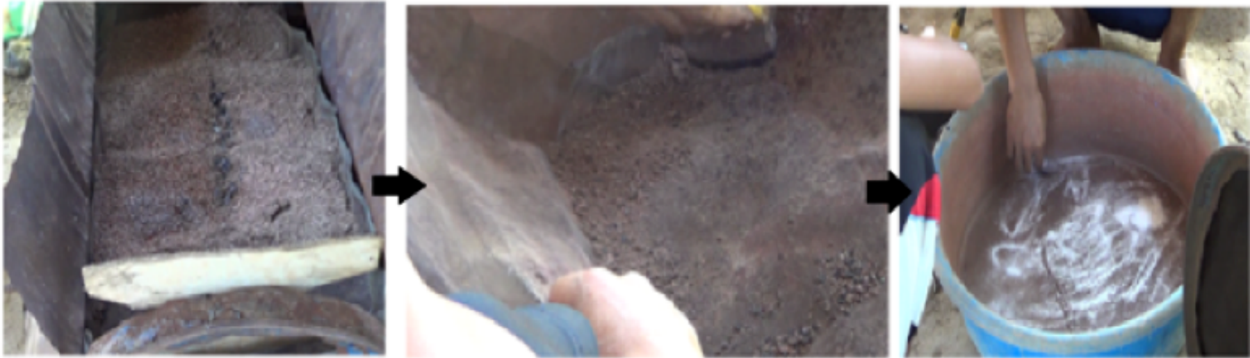
Figure 12. After burning with coco shell charcoal, the gold-loaded residue was captured using a mesh screen. Borax was then added.
