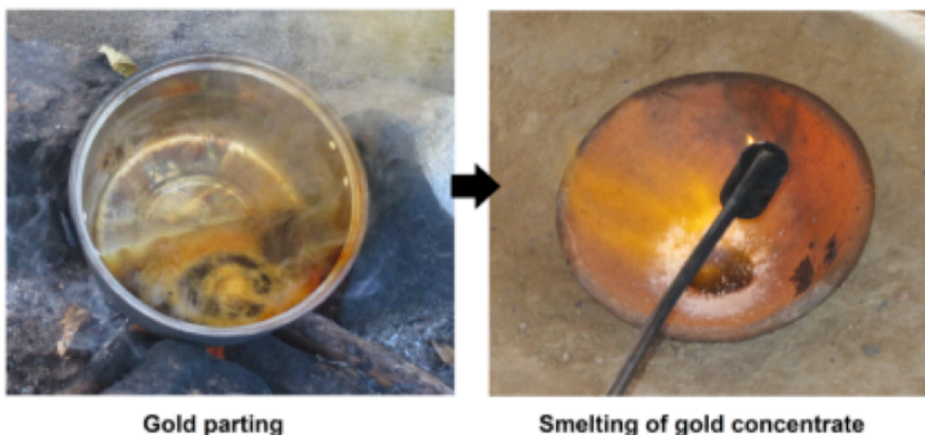
Figure 14. Heating with aqua valens and Smelting of gold concentrate
