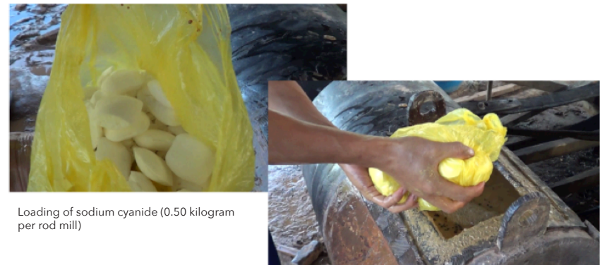
Figure 10. Addition of cyanide. Sodium cyanide (NaCN) is called puto-puto in the local community because of its semblance to the local rice cake.
