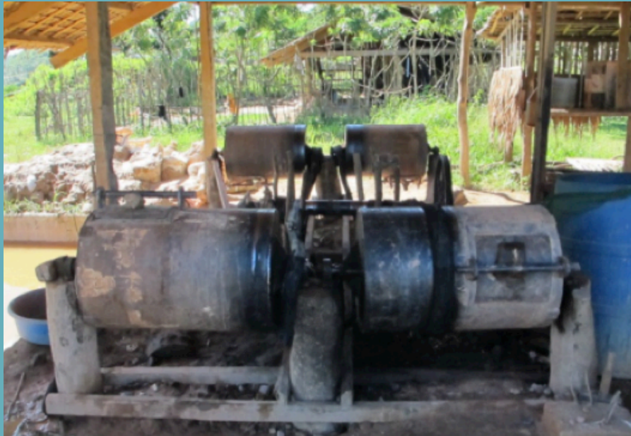
Figure 2. Small-scale mining facility which operates using the lugaw-lugaw (CID) process. This facility is composed of 4 rodmills attached to a single shaft by rubberized belts.
