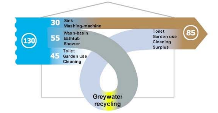
waste water recycling system
