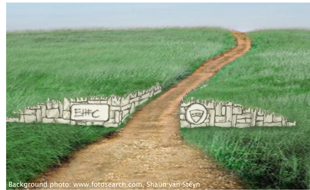
Board 3 2 The Gateway is designed to mimic a Ha-ha, which is a type of boundary used to control livestock, intended to not interrupt the view and to be invisible from close by.
