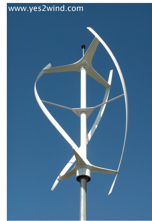
Board 3 3 The design of the Helical Wind Turbine allows power production with much lower wind speeds than the 3 blade wind turbine. Operating at lower wind speeds decreases noise and turbulence.
