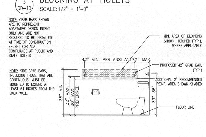
BLOCKING AT TOILETS MINIMUM BLOCKING REQUIREMENTS FOR ACCESSIBLE BATHROOM FACILITIES
