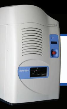
**The Echo 550** Compound Reformatter performs direct microplate-to-microplate transfers of droplets down to 5 nL using a new "touchless" transfer technology based on focused acoustic energy.
