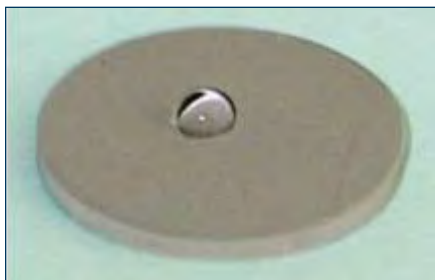
Figure 1 A drop of sterile saline is placed on the hydrophobic SLA® surface. The bead of water sits atop the SLA® surface due to the water contact angle of 139.9 degrees.
