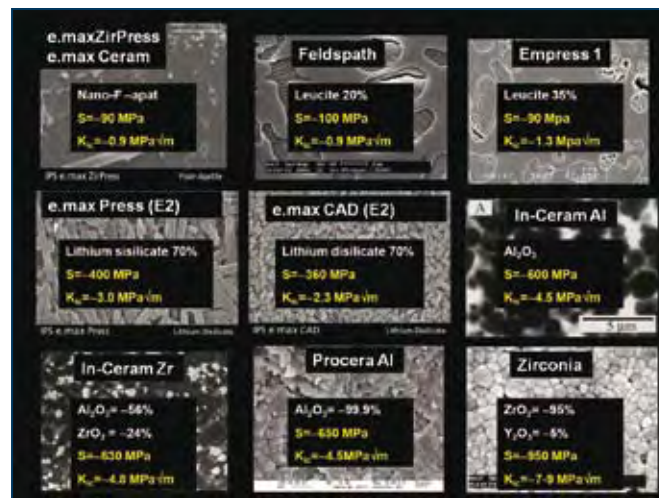
Figures 5a, 5b Scanning Electron Microscopy highlights the microstructure that gives strength to various ceramic restorative materials.
