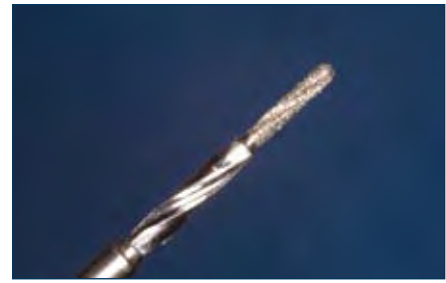
Figure 9 A close-up view of the diamond-tipped twist drill used to prepare the root for the extraction screw.
