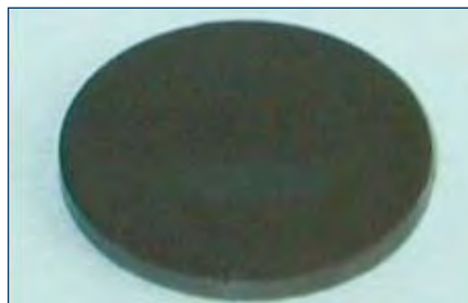
Figure 2 A bead of sterile saline is immediately absorbed into the chemically modified SLActive® surface. The SLActive® surface has a high surface free energy and is strongly hydrophilic, with a water contact angle of 0 degrees.
