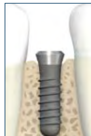
Figure 1 A view of a Straumann® soft-tissue level implant indicating vertical offset of the microgap from the crestal bone.
