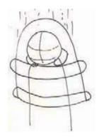
Adding ribs to the inflateable added strength and saved time and effort when blowing up. The final product would be easy to produce with ultra high frequency welding.
