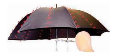
Wind tunnel testing of an existing umbrella informed not only the shape of our design, but also the materials and the way in which it would be held.
