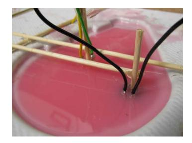
Each Pressure pad is moulded from soft silicone with a LED and a tactile switch imbedded. A force sensor is positioned underneath.
