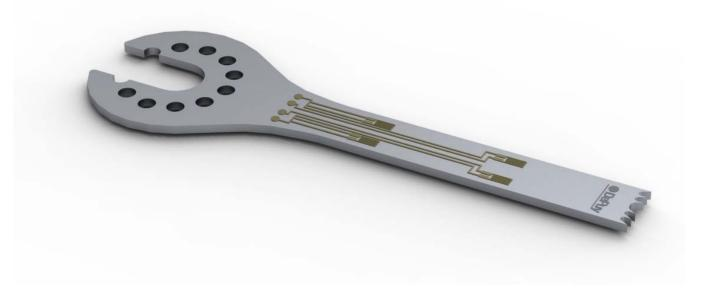
The use of strain gauges could greatly improve the accuracy of the system. In theory, if gauges were aligned as above, they could be used to detect only longitudinal strain. This can be used to calculate the bending of the blade, and visual feedback can be given to the surgeon.
