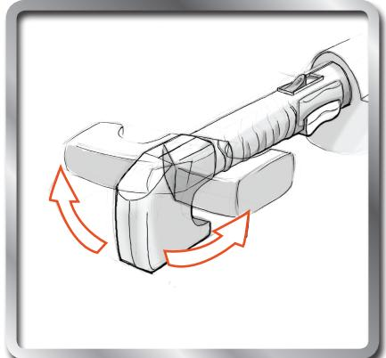
When the slide moves to the side, the handle is free to rotate to the side. This keeps the trigger in the same orientation no matter what side of the shrub is being trimmed.
