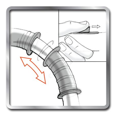
When the button on the rotating handle is engaged, the circle slide can move to the side. A notch in the circle keeps the slide at the top of the circle when not engaged for a standard grip.
