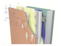
\* In this type of curtain wall the pressure-equalized system allows air to circulate behind the tiles of terra cotta through joints to provide a pressure-equalization in the cavity, which prevents water from entering into the interior walls, also along with a vapor barrier on the outside face that acts as a water barrier back ventilation which assists in maintaining a dry cavity and the buildup of hot air.
