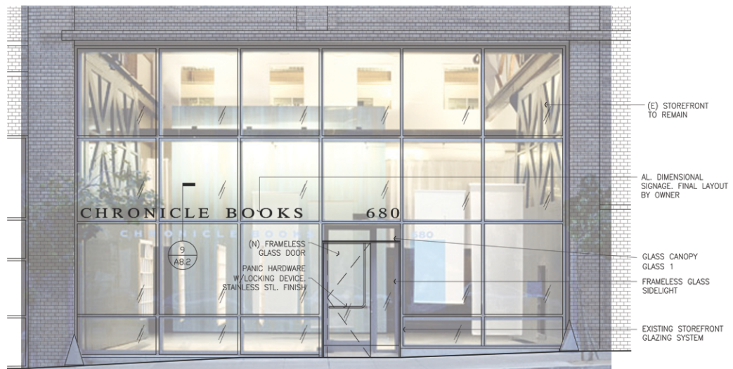
ENLARGED ELEVATION OF PROPOSED ENTRY 1/4" = 1'-0" ②
