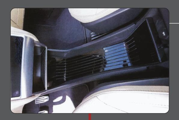
First, measurements were taken of the Tesla Model S's center space, and templates were made. The physical model's final measurements were then translated into a 3D model. That model then provided flat patterns from 3D curvatures, for CNC laser-cutting.
