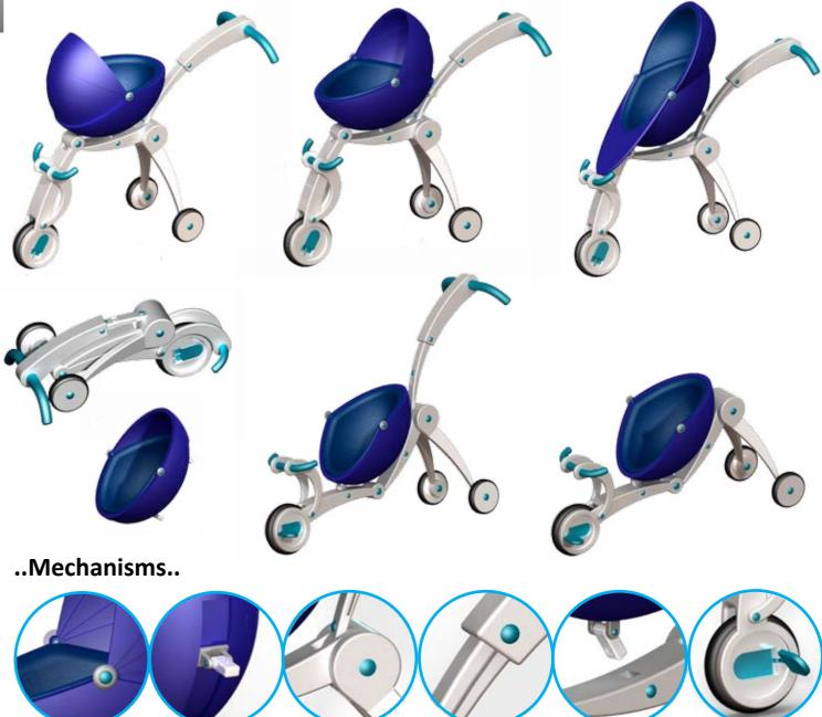
I designed the mechanisms to be the same throughout, using push release buttons to rotate/extend/attach parts.
