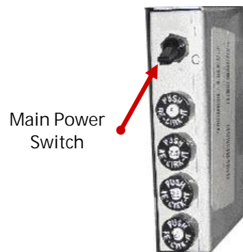
Figure 19: Turning Power On
