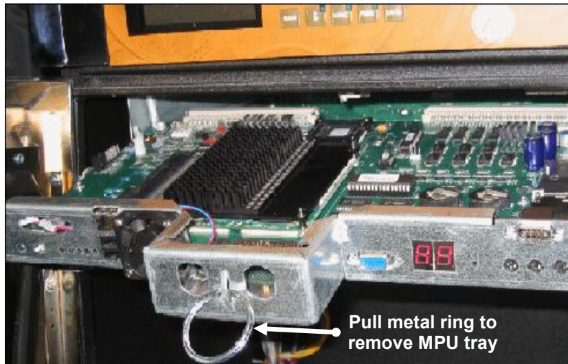
Figure 4: Removing MPU Tray
