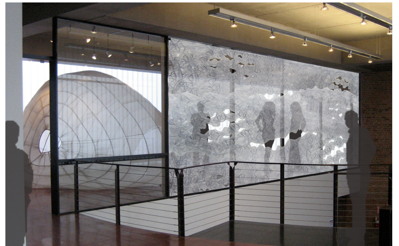
Early precedent material studies developed techniques of connection, aggregation, and performance. The vinyl tubing utilized its self-friction to form very sturdy connections through a looping and weaving technique. The entire fabric was able to grow in each of the axes by way of a system of offsetting the rhythm of the connections. This caused areas of separation where the level of transparency varied from near opacity to completely open apertures, creating an effect not entirely different than knot holes in wood fences.
