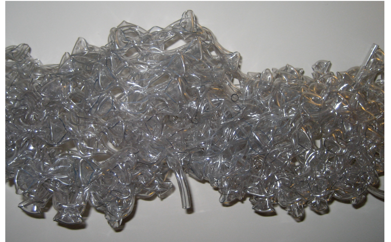
Early precedent material studies developed techniques of connection, aggregation, and performance. The vinyl tubing utilized its self-friction to form very sturdy connections through a looping and weaving technique. The entire fabric was able to grow in each of the axes by way of a system of offsetting the rhythm of the connections. This caused areas of separation where the level of transparency varied from near opacity to completely open apertures, creating an effect not entirely different than knot holes in wood fences.
