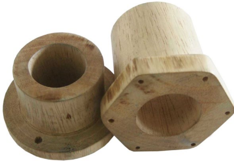
Rubber wood, manual lathe
