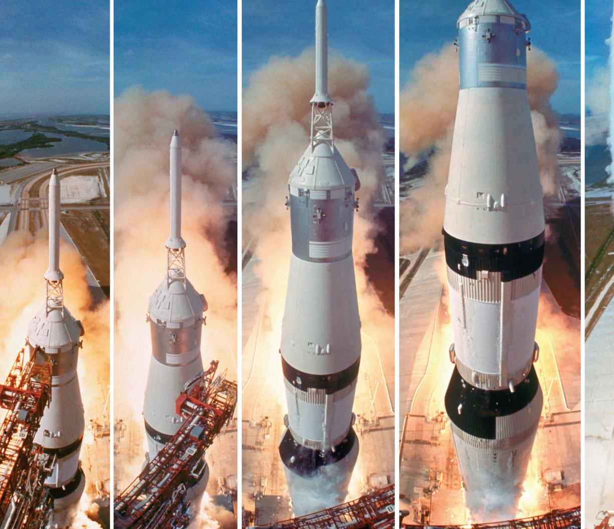
As the rocket boosters ignited and Apollo 11 began launching, the gantry (a bridgelike structure used for servicing the rocket) gradually disconnected, allowing the Saturn V to accelerate.
