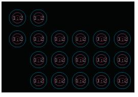
Fanouts also can be accomplished within Cadence SPECCTRA<sup>®</sup> for OrCAD using **Route > Pre route > Fanout**. Rules must be checked to be sure of the intended outcome. **Rules > PCB > General** has the setting to allow via-in-pad.
