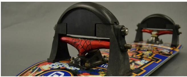
The 3D printed prototype deomonstrates the final form and part tolerances, while a pair of machined delrin protoypes demonstrate the function and strength of the final design.
