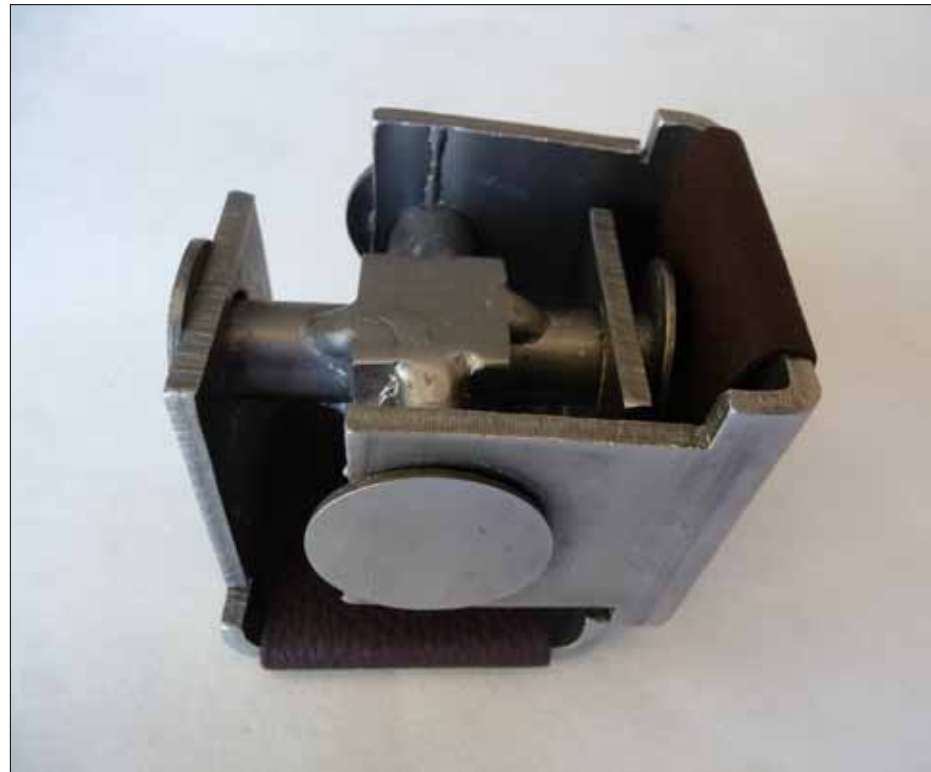
The final hinge was made of steel and leather. It is about 2 x 2 x 3 inches.
