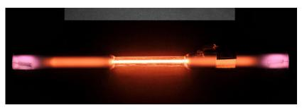
**Spark gap light-** consists of an arrangement of two conducting electrodes separated by a gap usually filled with a gas such as air, designed to allow an electric spark to pass between the conductors. When the voltage difference between the conductors exceeds the gap's breakdown voltage, a spark forms, ionizing the gas and drastically reducing its electrical resistance.
