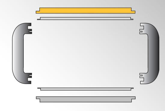
ABS sheet topper to give a good aesthetic look and a warmer feel than a full aluminium design, also could incorporate changes of colours due to user selection.
