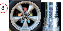
Tighten the lug nuts to the appropriate force as specified by the owners manual.
