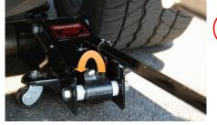
Loosen bleed valve slowly until the vehicle is back on ground. Let the jack release completely then remove from under vehicle.
