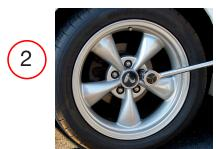
Loosen, but do NOT remove lug nuts from wheel.
