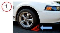
Put the vehicle in park or in gear and apply parking brake. Then place the wheel chocks firmly under the other tire on the same side.
