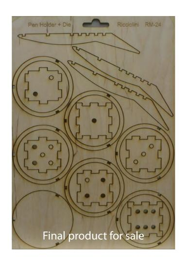
Cost of material: £1.02 Line lengh: 70.58cm Cutting time: 8m:23s Cutting cost/min: £0.25 Cutting cost: £2.06
