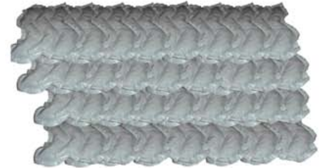
Garbage bricks as roofing
