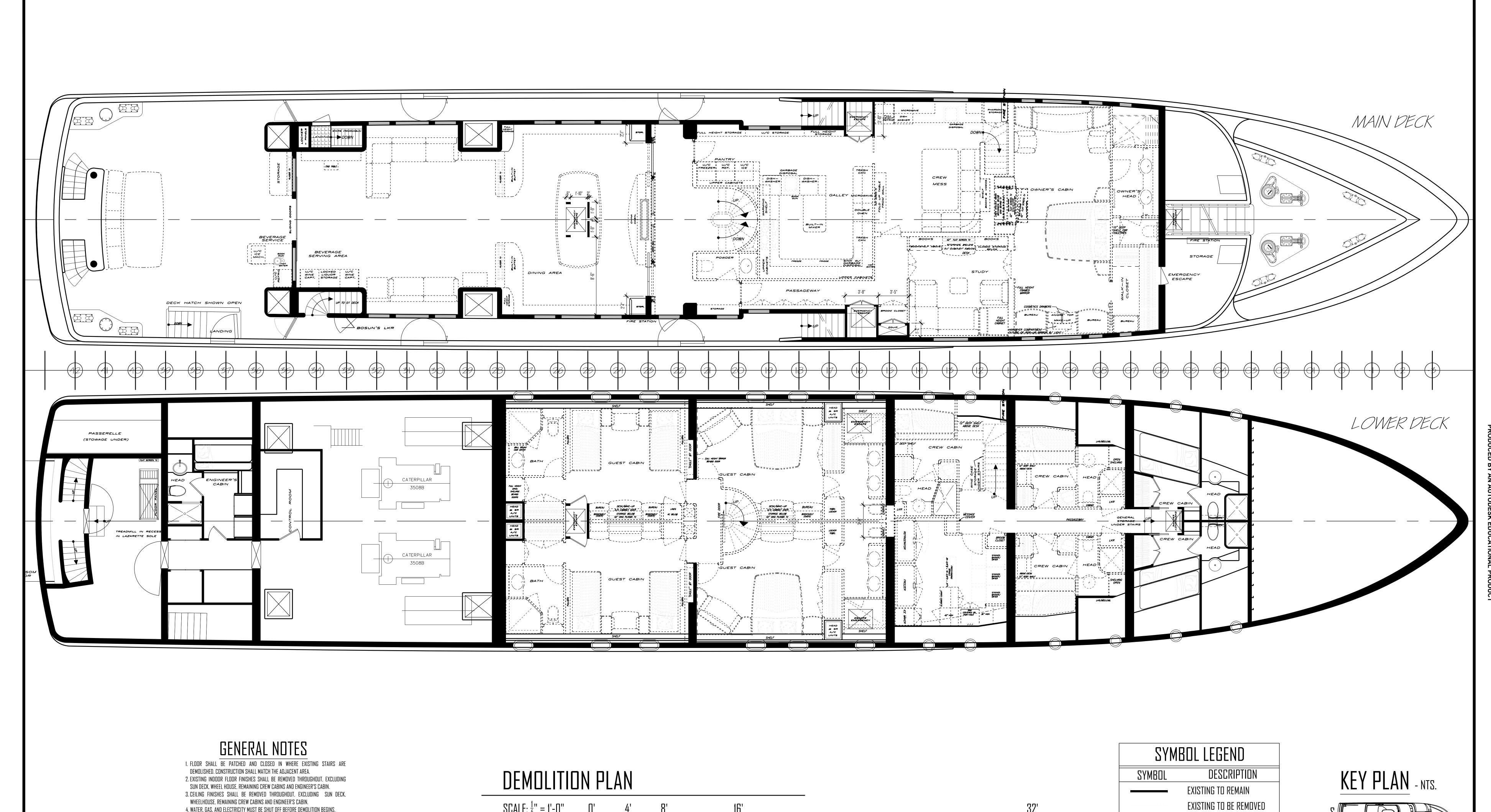
WHEELHOUSE, REMAINING CREW CABINS AND ENGINEER'S CABIN. 4. WATER, GAS, AND ELECTRICITY MUST BE SHUT OFF BEFORE DEMOLITION BEGINS. 5. PIPES AND DRAINS MUST BE PROTECTED BY PLUMBER BEFORE DEMOLITION BEGINS. 6. EXISTS MUST BE KEPT FREE OF OBSTRUCTIONS TO MAINTIN EXIT PATHS. 7. DUST MUST BE THOROUGHLY CLEANED OUT OF BOAT BEFORE AIR CONDITIONING IS POWERED ON AFTER DEMOLITION.
