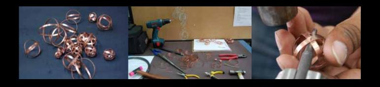
Skeleton of three dimensional heart made out of Brass wire and randomly create thin wire interlaced Structure on the surface. All the joint are covered with transparent resin, so that it won't hurt the wearer.
