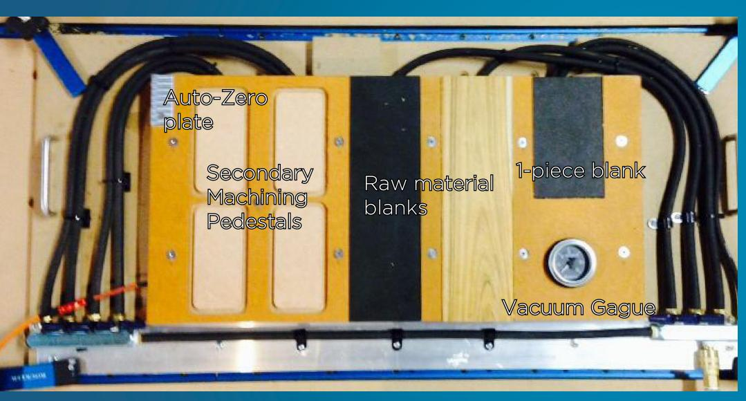
The second fixture is machined out of Richlite, the same recycled paper composite that the front face of the case is made from and holds a much stronger suction than the MDF.
