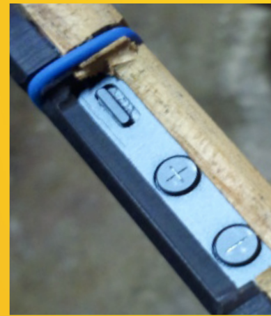
The key feature is an o-ring that holds the case together
