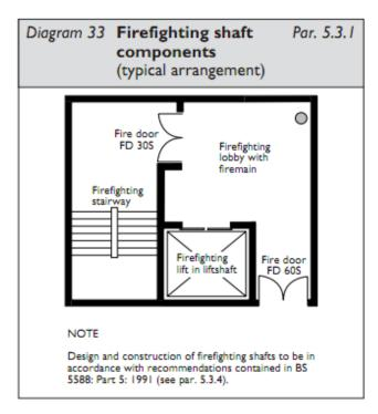
Note: All compartmentation walls and floors should have at least 30 minute fire resistance in accordance with the technical guidance documents
