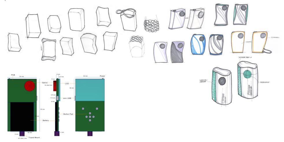
brief 1: develop two concepts for the company pyrma: the drome and pyrma drome hd cameras. drome hd should appear to be the 'pro' version of drome. all internals at set places and measurements, with requirements on logo size and placement.
