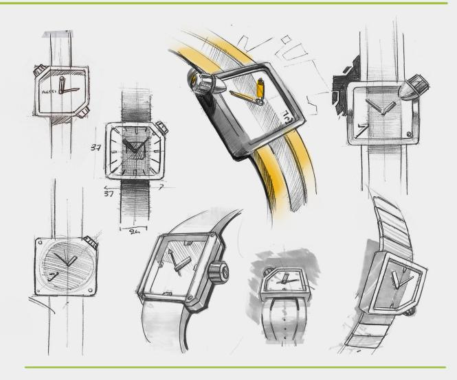
■ The crown is positioned on the top left part of the watch for ergonomic one hand winding and time setting.
