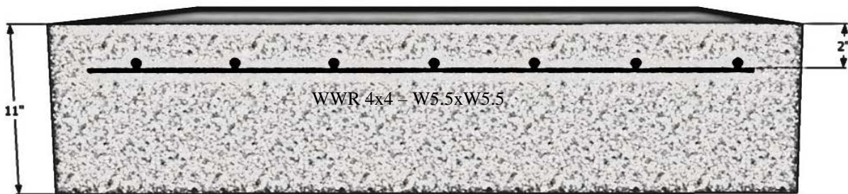
Figure S9: Slab on grade
