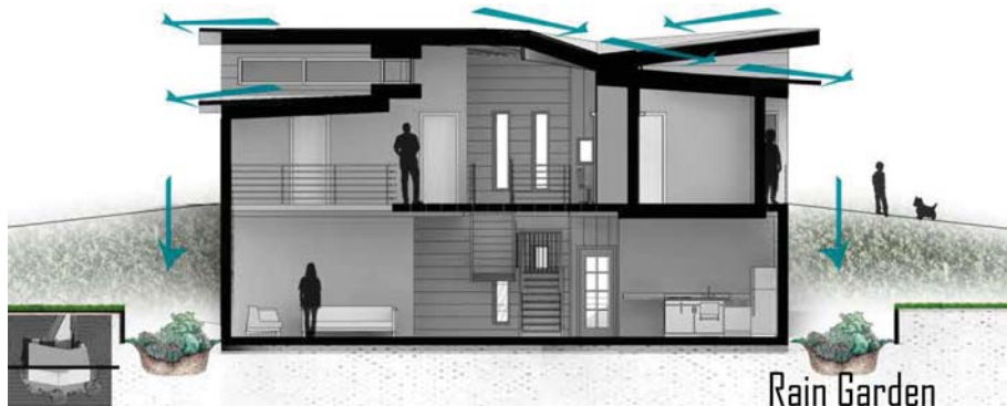
Roof angles designed to distribute water to rain gardens
