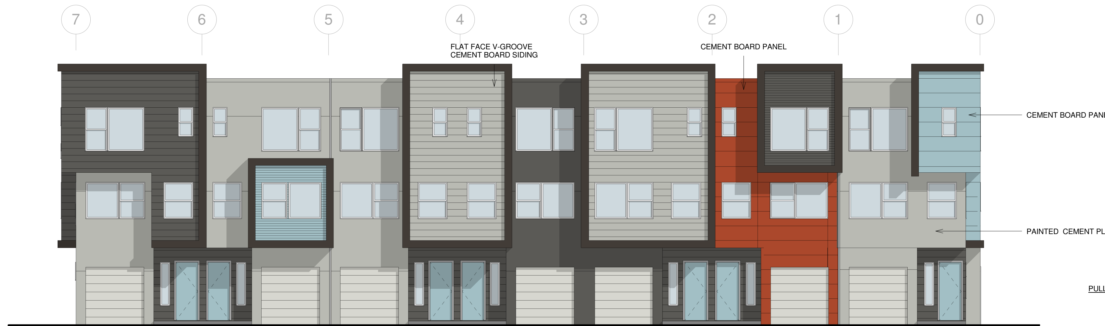
3 BUILDING 1 - EAST ELEVATION SCALE: 1/8" = 1'-0"
