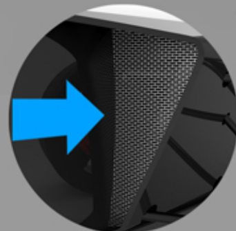
Radiator cooling intake duct
