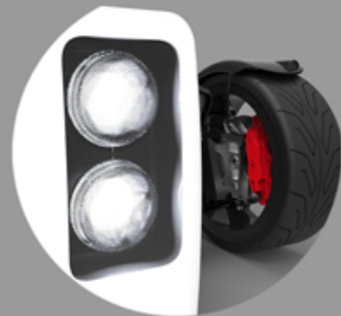
Central high and low beam lamps side indicators on wheel covers
