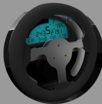
Motec SDL3 dash, aluminum sequential paddle shift, Momo steering wheel
